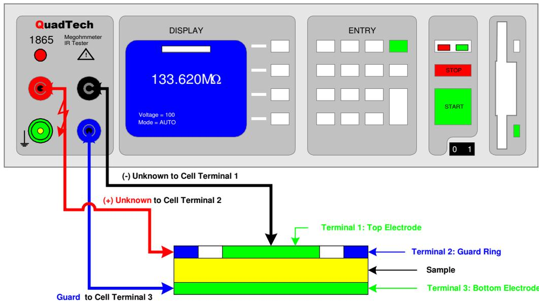
**Figure 2: Connection of 1865 Megohmmeter for Surface Resistivity Measurement**
