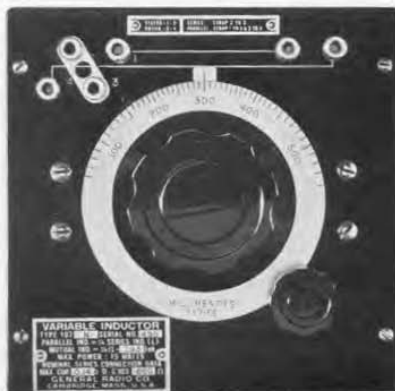
FIGURE 2. TYPE 107 Variable Inductor. Mutual inductance at any setting is one-half the difference of the scale reading and the value of self-inductance at zero mutual inductance as entered on the nameplate
