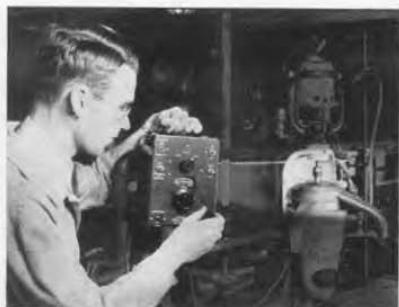
The TYPE 631-A Strobotac as used to measure the speed of a centrifuge
