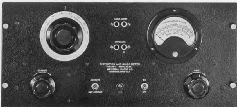
Panel view of the Distortion and Noise Meter. Note the open, easily-read scales. Full-scale ranges of 1%, 3%, 10%, and 30% are provided
