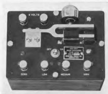
FIGURE 1. This electro-mechanical oscillator operates at 1000 cycles on power from 6 volts, direct current. The output circuit is a tapped transformer
