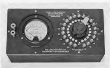
FIGURE 2. When bridged across the line, voltmeter fashion, this instrument indicates the amount of power that is being delivered to the 500-ohm line beyond the bridging point. It is direct-reading in decibels for a zero level of 6 milliwatts
