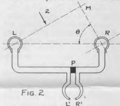
ily be located close to the rubber receivers in order that the sound energy shall not be unduly attenuated in passing through long pipes. Such a location on shipboard is frequently inconvenient as well as uncomfortable for the operator.
