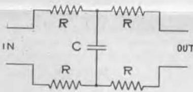
The loop resistance  $4R$  and the shunt capacitance  $C$  of the section are made the same ratio as the loop resistance and shunt capacitance of any given length, say a mile, of the type of cable in question.
